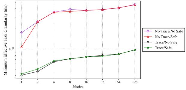
Figure 21. METG(50%) overhead of control determinism checks, both with and without tracing (lower is better).
