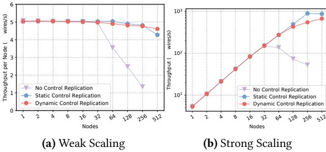
Figure 13. Scaling of Circuit Simulation Benchmark.
