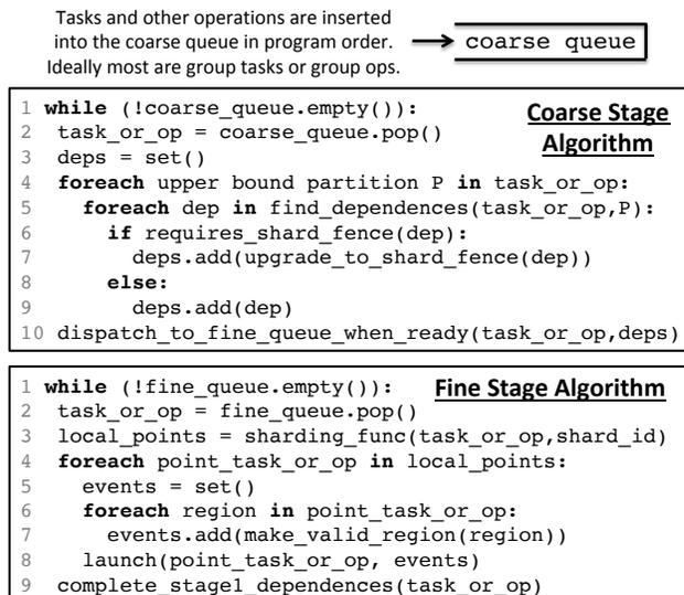
**Figure 9.** Pseudo-code for the dependence analysis algorithm. Each stage operates independently and continuously on every shard for the lifetime of a DCR program.
