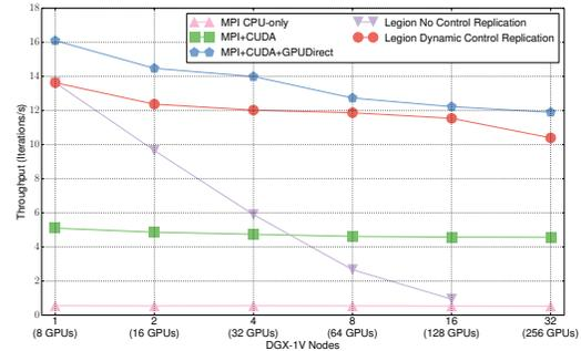
Figure 14. Weak scaling of Pennant compared to MPI.
