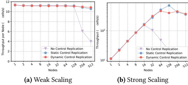
Figure 12. Scaling of 2D Stencil Benchmark.
