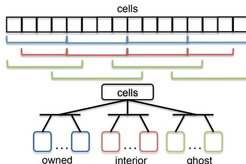
Figure 8. A region tree with three partitions to describe different subsets of cells used by different tasks in the stencil example. Ranges of sub-regions are depicted visually at top.
