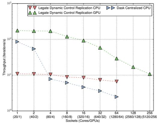
Figure 20. Preconditioned CG Solver in Legate NumPy.
