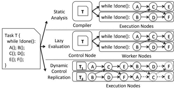
**Figure 1.** Approaches to implicit parallelism: static analysis and lazy evaluation centralize analysis and distribute partitioned programs to workers for execution. DCR executes a replicated program, dynamically assigns tasks to shards, and performs an on-the-fly distributed dependence analysis.
