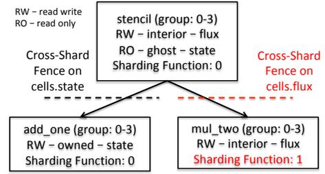
**Figure 11.** Changed dependence analysis (in red) from an alternate selection of sharding function for `mul_two`.
