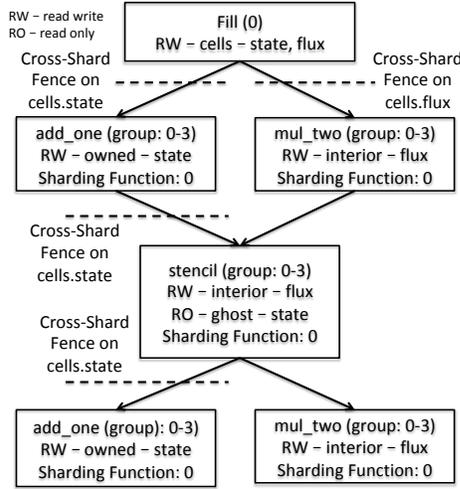
**Figure 10.** Coarse stage dependence analysis computed by every shard for the program in Figure 7.
